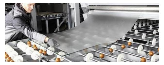
Then the upper sheet is placed and the sandwich is complete. This sandwich is prepared in a prelaminating process for the subsequent auto-claving process. In the autoclave the sandwiches are finished under vacuum and heat. The air is extracted from the sandwich laminate, the PVB foil melts and combines with the glass to form a laminate.
