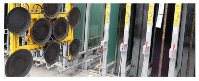
Simple handling devices for manual loading usually consist of several vacuum suction cups attached to one design (see picture above). If the vacuum suction cups are arranged too tightly, central stress is created during the lifting process. A lifting device with vacuum suction arms that distribute the lifting forces over the entire surface should be preferred.
