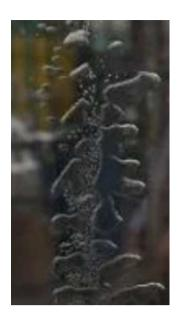
If too much heat is applied in pre-lamination, the foil becomes sticky and the air that is present cannot be properly pressed out of the glass package.
