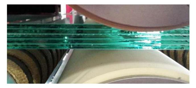
The pressure that is needed is applied to the warm glass package with the heated foil via the rollers in order to achieve the initial adhesion between the foil and the glass, and press the air out of the laminated glass sandwich.
