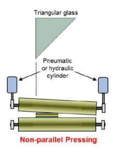
The hydraulic or pneumatic press is used by the majority of suppliers because the cost is lower, but the disadvantages cannot be dismissed out of hand.
