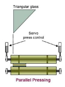
On the other hand, pressing force application using spindle technology is known to be very precise. Because the tolerance margin with this technology is very small in contrast to hydraulic and pneumatic press force application, and takes place within the range of tenths.
