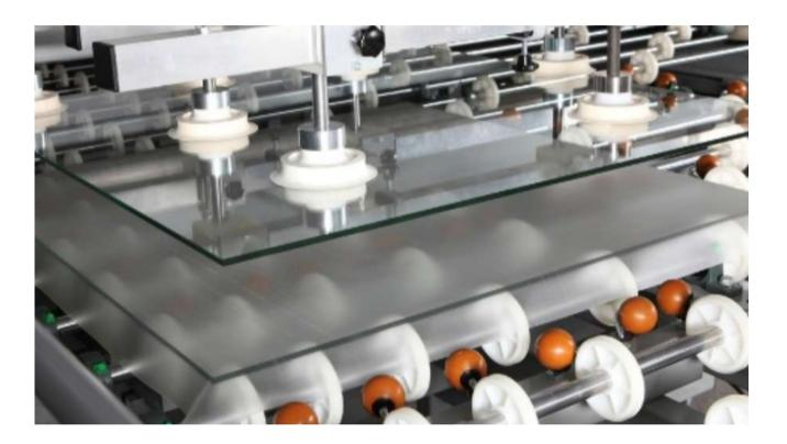
Glass alignment is the real "bottleneck" of a lamination system. The converter places the aligned glass onto the first glass and the foil. The availability of the glass sheets is particularly important when it comes to production speed with this process.
