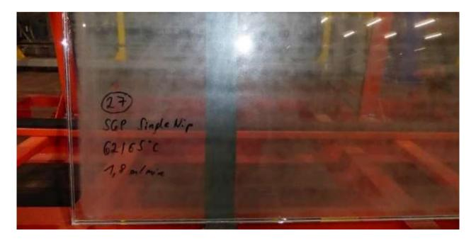
On the other hand, the foil structure is still visible in the remainder of the laminate. It should appear even across the entire area. This shows that the pressing force of the pressing rollers and heating by means of convection or radiant heaters were always good and even during lamination.
