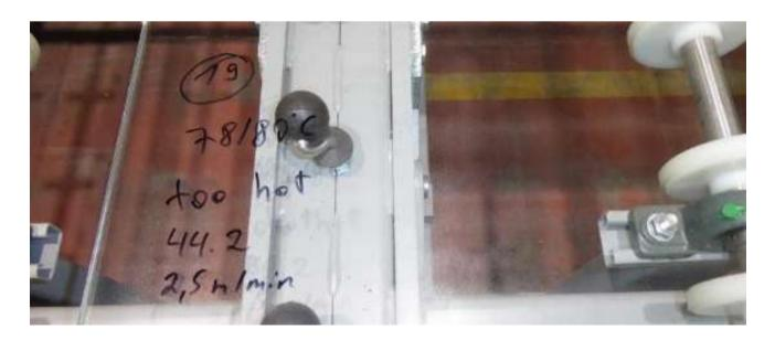
This residual air expands in the autoclave or additional air is pressed into the laminate due to the lack of foil adhesion to the glass and the 12 bar of overpressure. This creates many circular bubbles, and the glass package does not appear transparent as it should.
