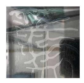
Improper storage of the foil, resulting in the moisture content being too high, can also lead to delamination. The adhesion between the glass and the foil is therefore reduced, which can either lead to the first signs of delamination after the autoclave, which are evident from round bubbles (ice flowers) - or not until the product has been used in a façade, for example. However, the quality of the "gluing" is also reduced in this case.
